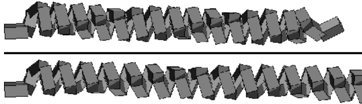
Figure 19: A sequence of images from region III in the simulation. All the layer to layer bonds have broken. Further elongation now comes from the stretching of the pairwise bindings.
