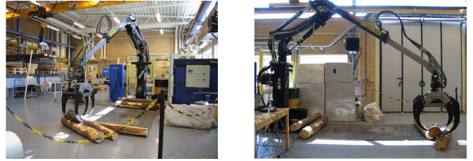
Figure 4: The forwarder crane of reduced size at Smart Crane Lab.
