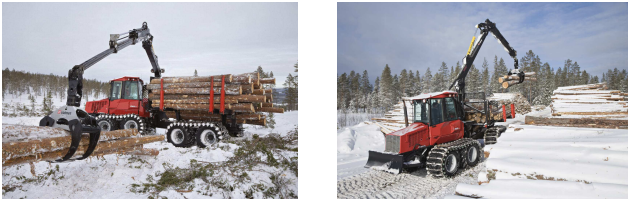
Figure 1: Large-scale manipulator on forwarder machine (Valmet 860.4) loading logs at the felling site and unloading at the road side. Image courtesy of Komatsu Forest.
