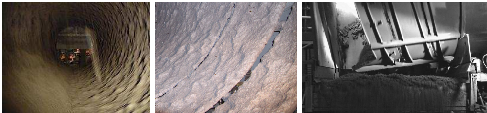
Figure 9: Sample images of drum interior (left and middle) and distribution on wide-belt conveyor (right). The bulk flow of ore pellets circulate in the lower left section of the drum. The fine material adhere to the drum walls and form an irregular surface coating. The middle image show a close-up of the irregular drum surface and coating of fine material around the outlet gaps.
