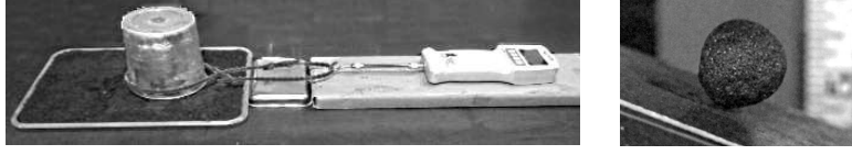
Figure 5: Measurement of surface friction (left) and rolling resistance (right).
