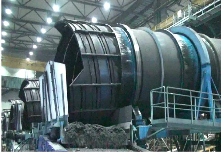
Fig. 1: A balling plant showing part of the balling drum, outlet, belt conveyor and roller screen. Picture courtesy of LKAB.
