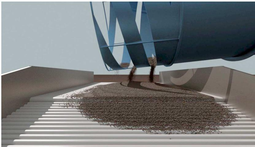
Fig. 4: Capture from simulation showing material flow from the outlet onto the conveyor and roller screen.
