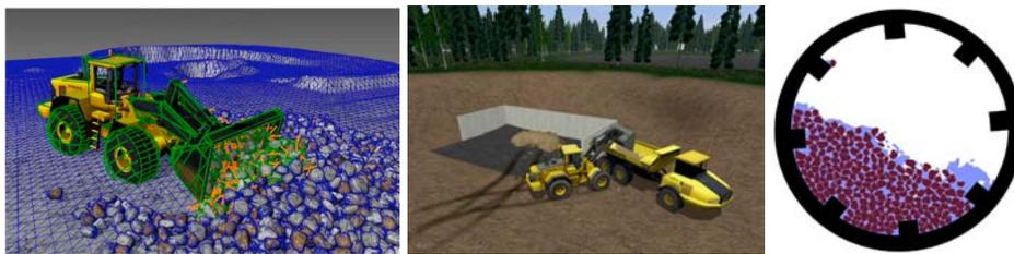
Fig 3. Image from prototype system, final wheel loader simulator and samples from simulation involving a mix of rigid particles and SPH fluid.
