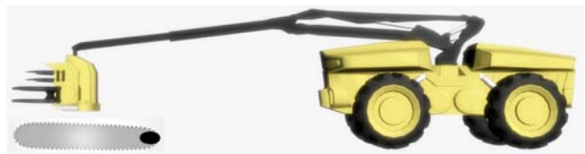
Figure 2. Illustration of the machine concept for harvesting in young dense forest stands. The machine is unmanned, semi-autonomous and operated remotely. The harvester may be equipped with a single tree harvesting head, a conventional accumulating multi-tree harvester head or a harvester head with long chainsaw sword for corridor harvesting.
