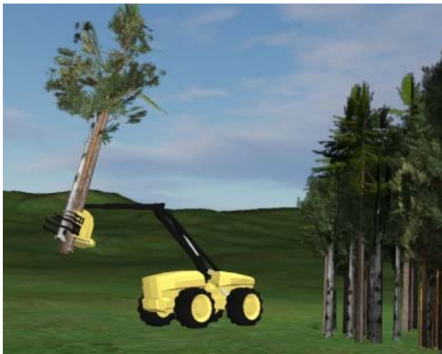
Figure 4. Snapshot from simulation. The machine is gripping several trees with a multi-tree harvester head.
