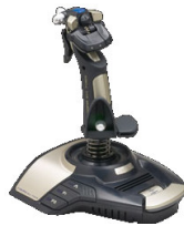
Figure 5.4: A gaming joystick with force feedback support from Saitek.
