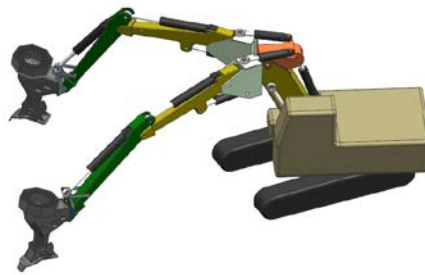
Figure 2. The two-armed excavator base machine model.
