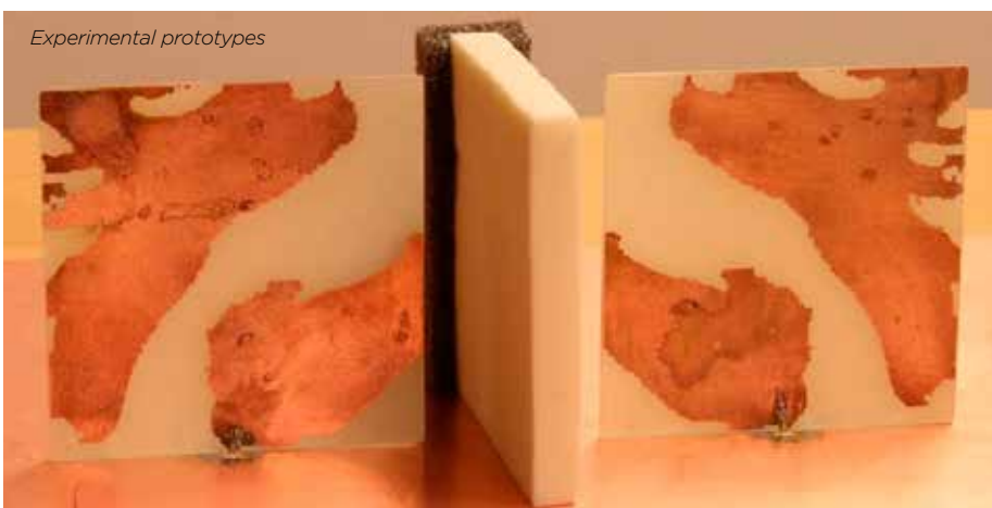
A pair of microwave antennas on printed circuit boards optimized for nearfield sensing and communication. The device could be used, for instance, for noninvasive monitoring of bone regeneration and healing.
